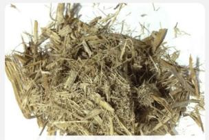
Bagasse (fibrous residue that is left over as a waste product when the juice has been pressed out of the sugar cane)
