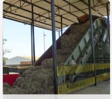
Bagasse is moved on a conveyor belt to the baler
